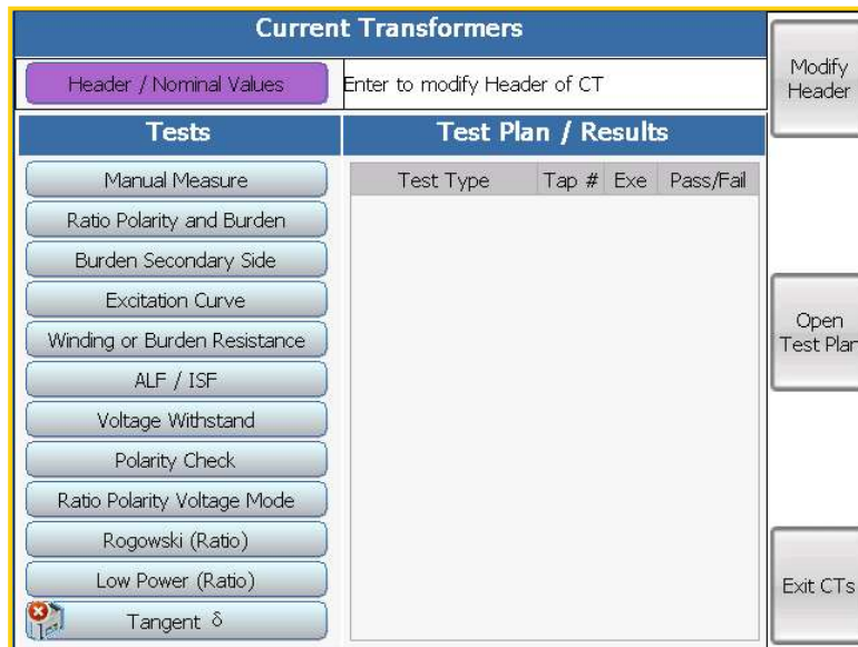
Figure 11 - "Current Transformers" test page (Conventional Type)
