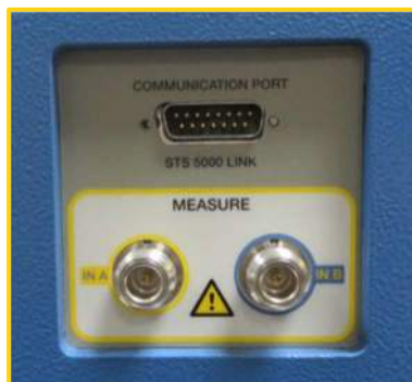
Figure 35 - IN-A (UST-A) and IN-B (UST-B) measurements on the side
