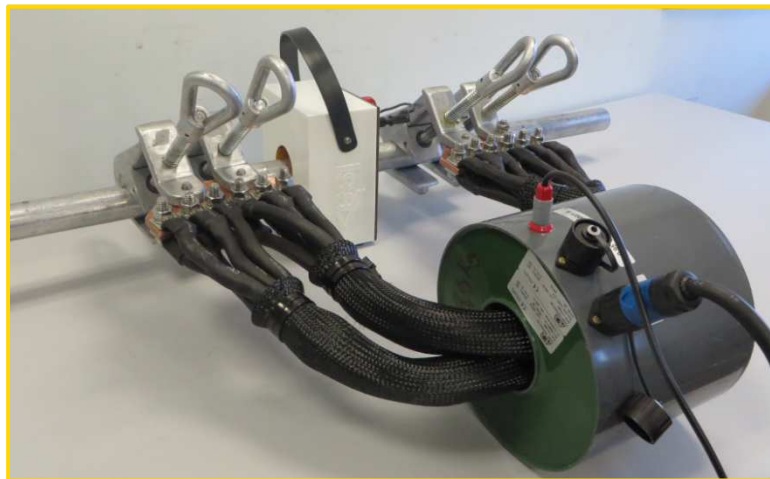
Figure 22 - BUX 5000 option connected to a CT under test
