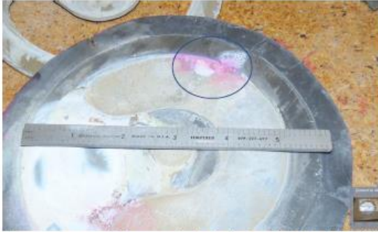
Figure 10 Arrester top diaphragm outside showing location of crack found with red die. .
