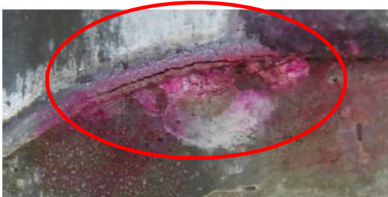
Figure 10 Arrester top diaphragm outside showing location of crack found with red die. .
