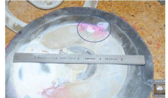
Figure 10 Arrester top diaphragm outside showing location of crack found with red die.
