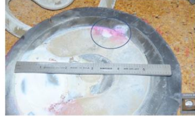
Figure 10 Arrester top diaphragm outside showing location of crack found with red die.
