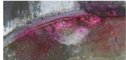
Red dye penetrated through the top diaphragm.
