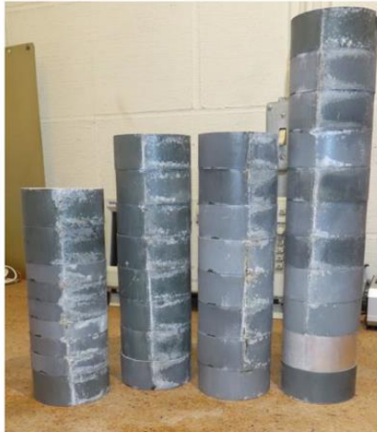
Electrical tracking along the MOV Blocks
