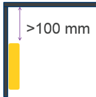
Figure 21: Keep Air Interface away from nearby metals
