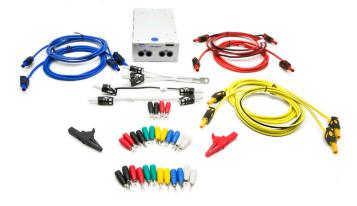
The HVA Current Module provides two 25 A sources at 150 VA each. When both sources are connected in parallel, 50 A at 300 VA continuous power is produced. Transient mode enhances the ratings of the HVA Current Module which extends the range up to 90 A at 300 VA for 30 seconds. DC output is 50 A.
