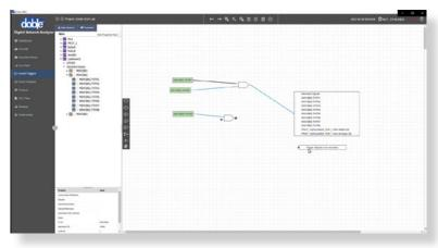
Set DNA triggers to record data prior to and following events. The captured data is scanned to produce an Event Analysis Report.
